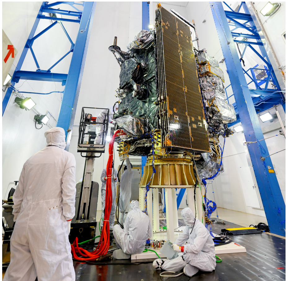
GOES-U acoustics testing. Photo credit: Lockheed Martin
