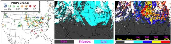
Figure 4: Left: Icing PIREPS on Nov. 8, 2008. The Flight Icing Threat icing mask (Center) and icing intensity (Right) are shown, derived from current GOES at 1745 UTC on Nov. 8, 2008. Icing intensity is expressed as the probability of encountering light (LGT) or moderate or greater (MOG) icing.
