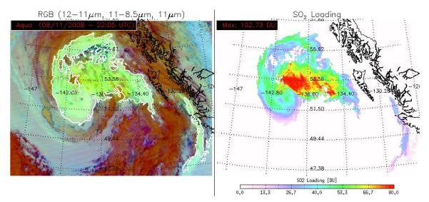
Figure 5: Example GOES-R SO2 products generated using Aqua MODIS data from August 11, 2008 at 22:05 UTC. The SO2 cloud present in this scene is from an eruption of Kasatochi, located in the Aleutian Islands of Alaska. A false color image (left panel) and the estimated SO2 loading (right panel) are shown. The SO2 detection results are displayed as white contours on the false color image.
