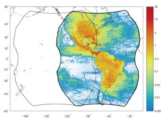
GLM coverage from the operational GOES East and GOES West positions, populated with the first nine months of lightning flash density observations from the GOES East GLM. The flash density is plotted for 2017 December -2018 August within units of flashes per square km per month. Credit: NOAA
