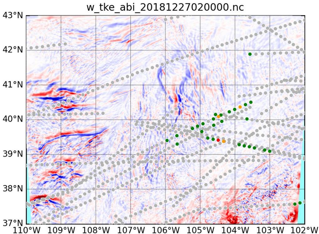
*Figure 3. WRF-derived Turbulent Kinetic Energy (colormap) and corresponding aircraft EDR (plotted points) for one of the modeled cases.*
