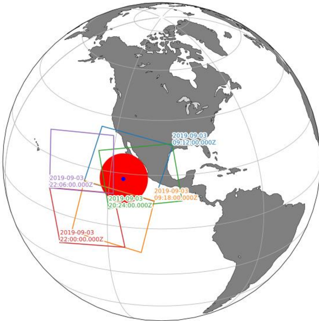
Figure 1. JPSS1 VIIRS 6-minute granules within 1000km of east Pacific Hurricane Juliette (2019), centered at 18.2°N, 114.7°W between 2019-09-03 00Z and 2019-09-04 00Z. Shown are both Day and Night Passes
