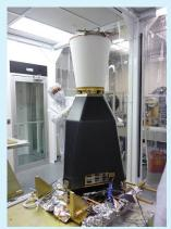
GLM is the first operational lightning mapper flown in geostationary orbit and measures total lightning (in-cloud and cloud-to-ground) activity. GLM collects information such as the frequency, location, and extent of lightning discharges to identify intensifying thunderstorms and tropical cyclones. Intensifying storms often exhibit a significant increase in lightning activity.
