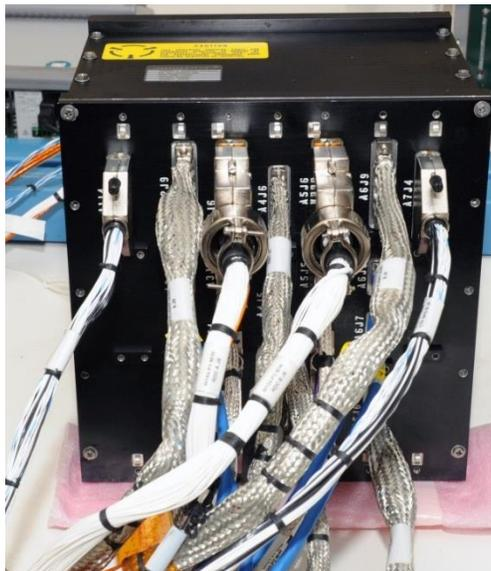
**Figure 10-2. The Command and Telemetry Processor (CTP)**
