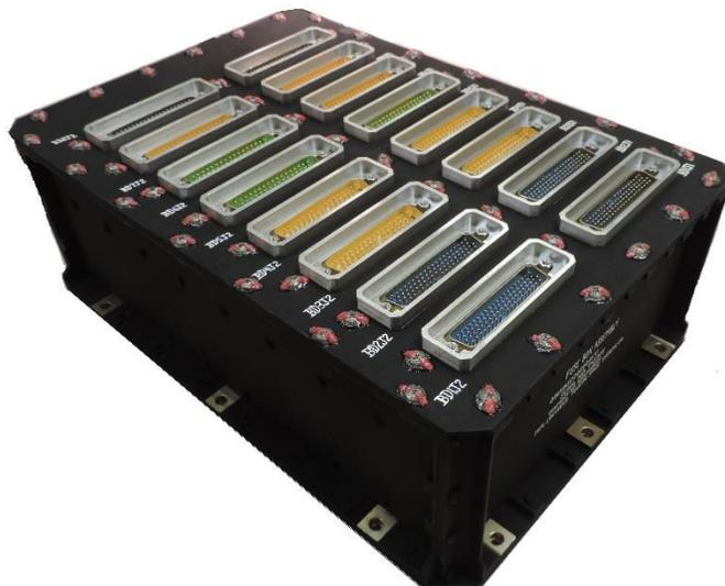
**Figure 11-8. A Fuse Board Assembly**
