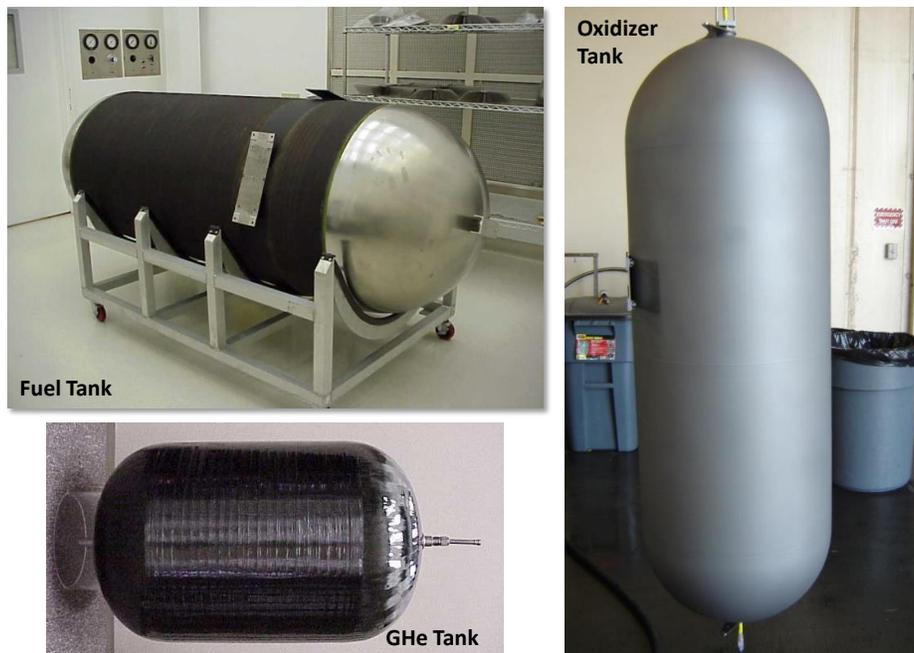
**Figure 13-3. GOES-R Series Spacecraft Propellant and Pressurant Tanks**
