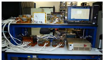
The Extreme Ultraviolet X-Ray Irradiance Sensor (EXIS) FM1 successfully completed of all post-environmental calibration activities in March. The instrument was transported to Goddard Magnetic facility where it completed the powered-off magnetic testing.
